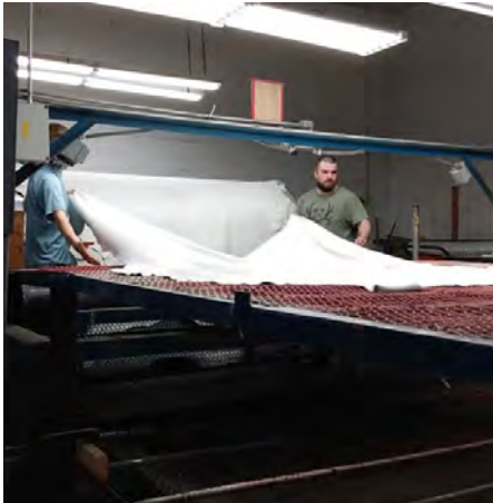
Working together to pull the hides off the sprayline after being stuccoed and getting them up on the horse. Great work team!
