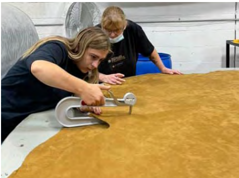
Barb Knowles working with Paige Coyle measuring the thickness of the larger cow sides.
