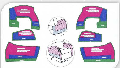
Each hide goes through a complete inspection. The inspectors grade the hides including different zones to identify each characteristic of every hide. This procedure is a 3 step process.
