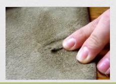
Step 2 includes pulling the leather over foam to give an upholstered look. This step allows the inspector to view the leather in depth. The foam allows you to see imperfections that you didn't see in step one.
